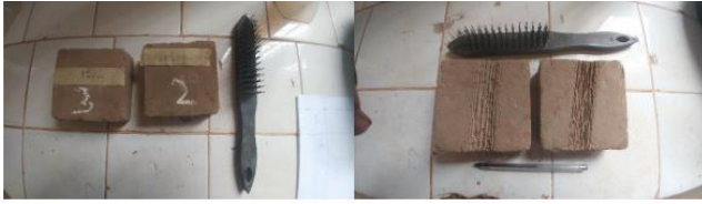
Figure 8. Abrasion test.
